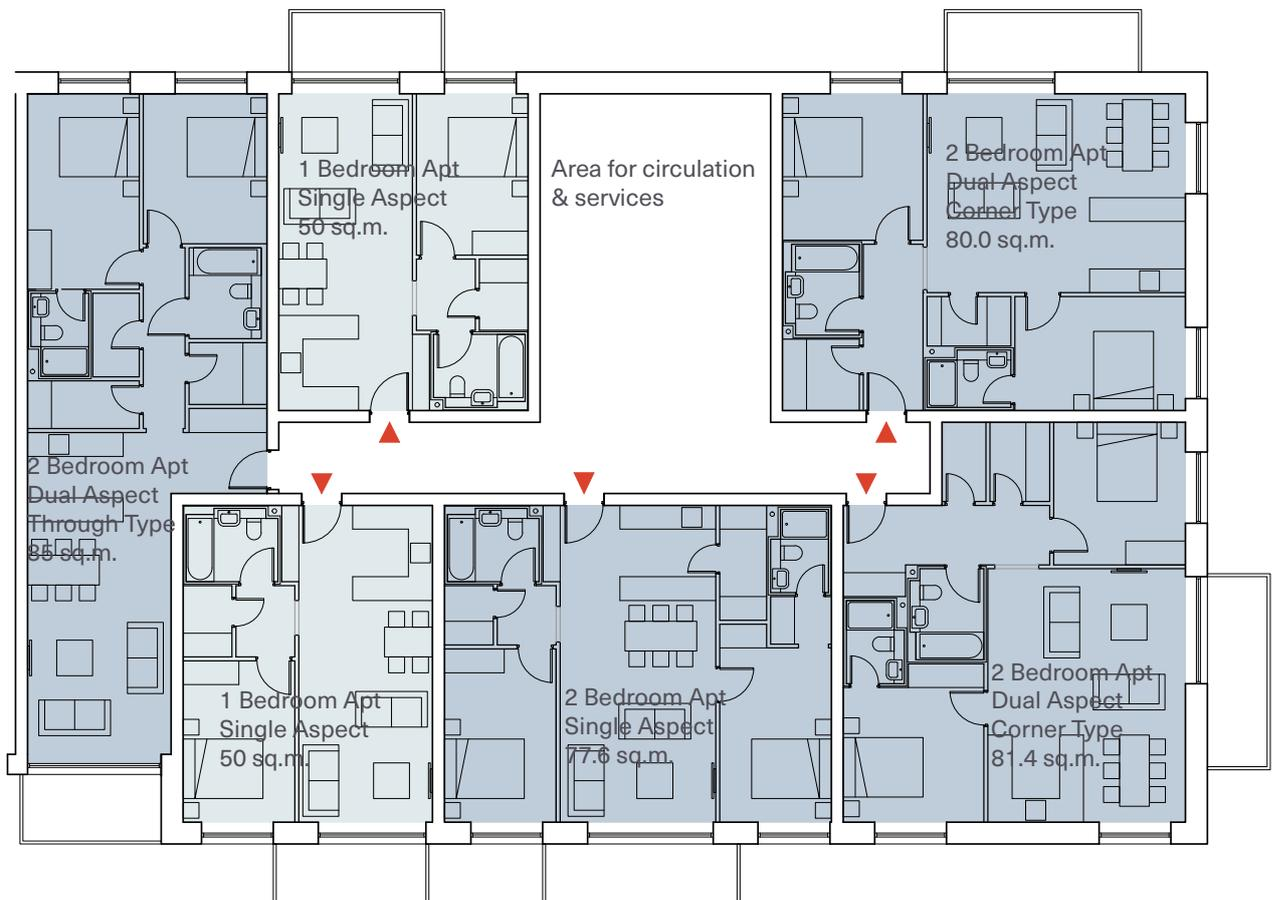
**Diagram 1:** Typical arrangement of an apartment building, with 8.0 metre deep unit types, which would generally achieve compliance with the BR209 (BRE Guide) standards. All units shown are compliant with the Design Standards for New Apartments 2020.
